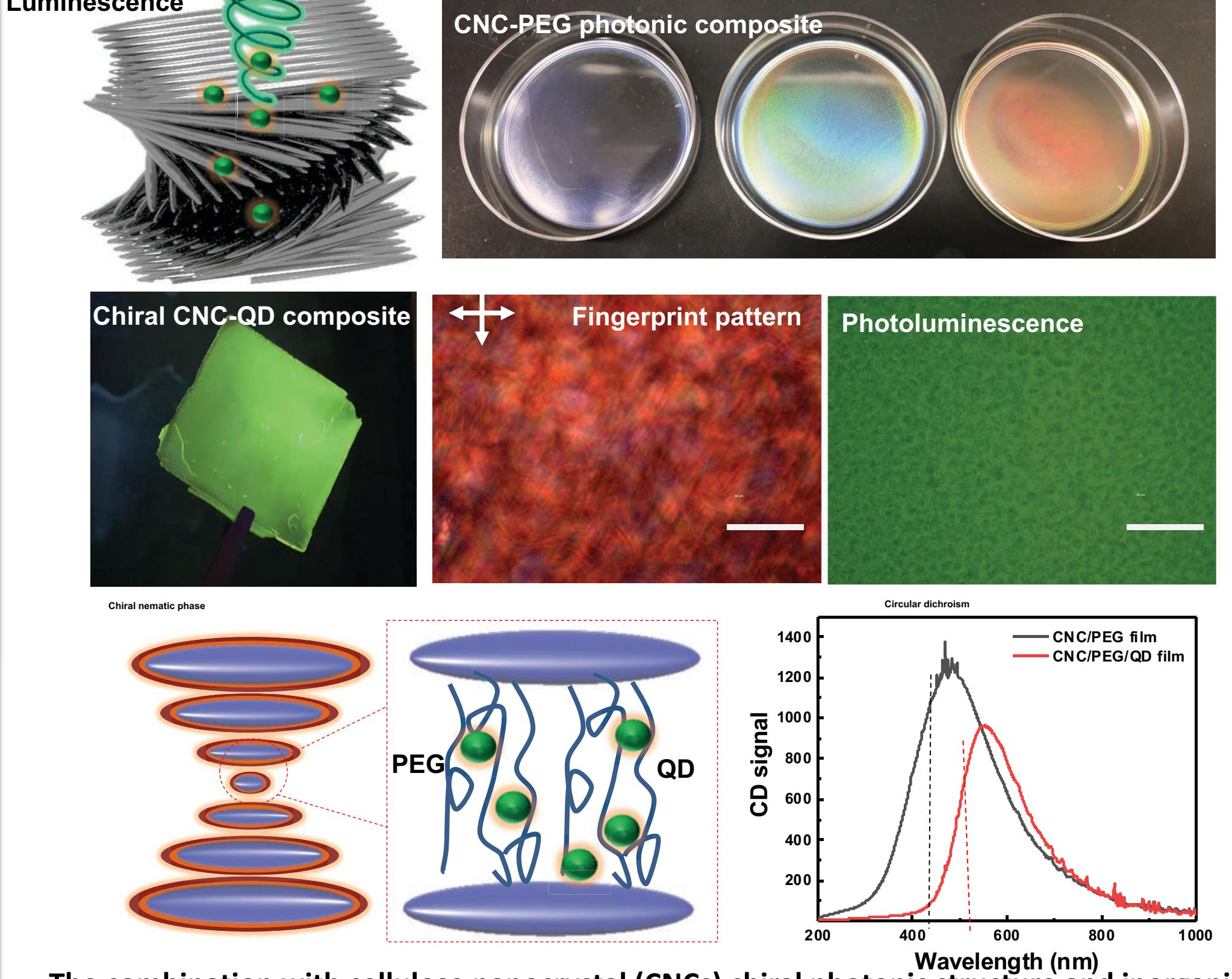
The combination with cellulose nanocrystal (CNCs) chiral photonic structure and inorganic quantum dot (QD) with achiral morphology provides well-designed chiral photoluminescence with strong circular dichroism (CD) peaks without destroying initial chiral nematic phase of CNCs.
